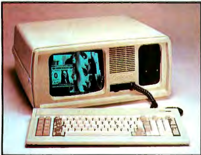
Photo 1: The Corona Portable PC, a portable IBM PC clone with a high-contrast display.
