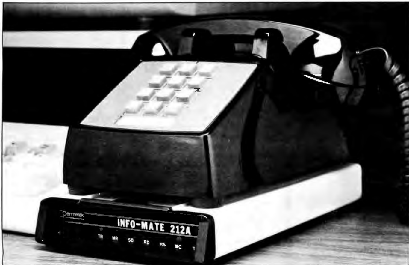
Photo 1: A command-driven auto-dial, auto-answer modem (Cermetek's Info-Mate 212A).
