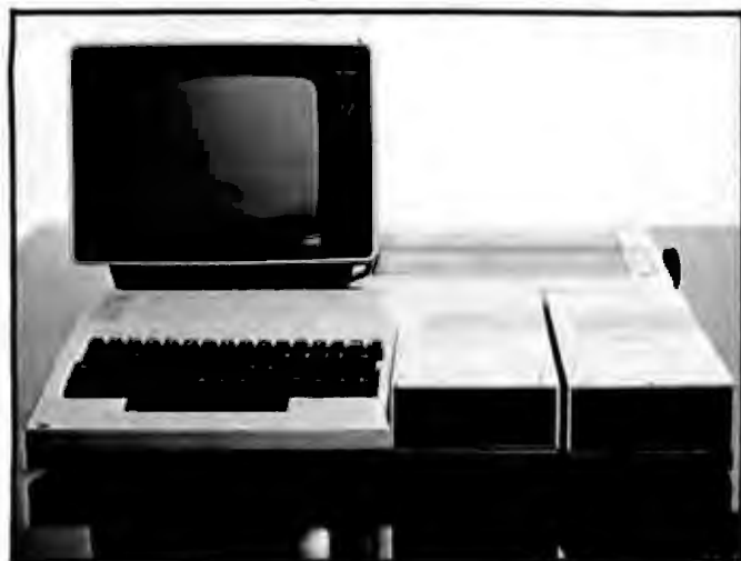
Photo 1: A prototype Pied Piper portable computer with optional second disk drive, monitor, and printer.
