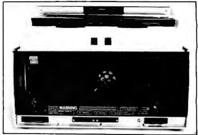
Photo 5: The rear panel of the Access showing (left to right, top): power cord storage compartment, on/off switch, and fan. Bottom panel (left to right): bidirectional parallel port, two RS-232C serial ports, external video monitor jack, and IEEE-488 port.
