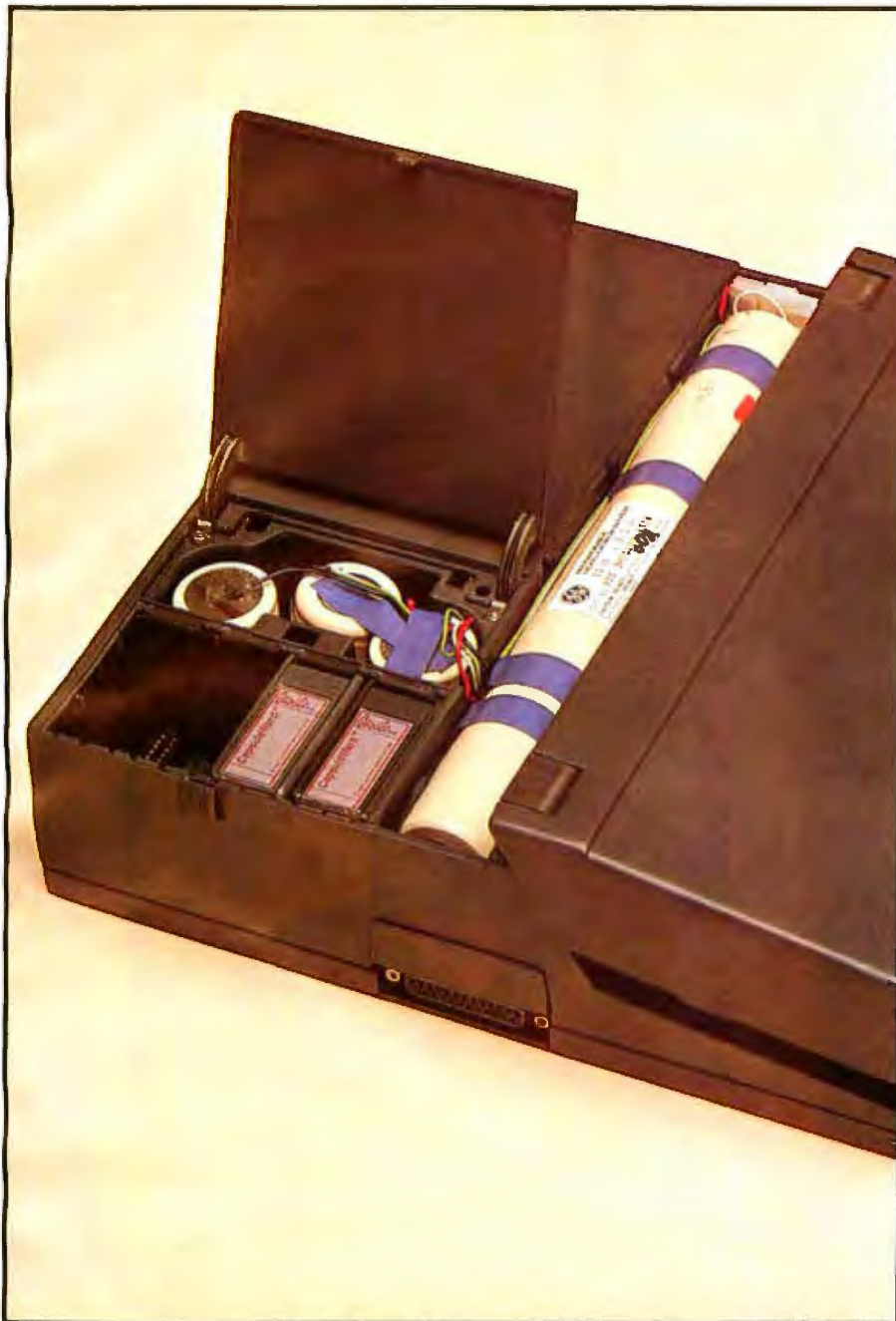
Photo 4: The battery pack consists of 10 1/2-D nickel-cadmium cells, seven of which are in tubular form beside the disk drive and memory capsule enclosure. The remaining cells are housed side by side in an upright position in the space between the disk drive and the capsule enclosure.
