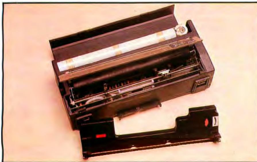
Photo 6: To conserve space and minimize power consumption, a thermal print head is used. Unlike other thermal printers, however, the Gavilan printer prints on plain paper. The key is a special thermal transfer ribbon contained in a pop-out cartridge, which can be removed when thermal paper is used.
