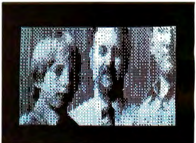
Photo 2b: The Apple II's display represents gray levels as different densities of white dots. Several different-length exposures are combined to form the gray-scale image.
