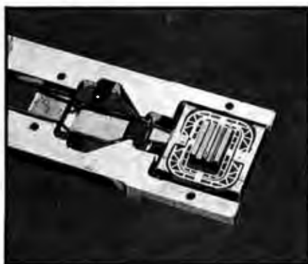
Photo 1: The read/write head assembly developed for DMA's fixed/removable hard drives.
