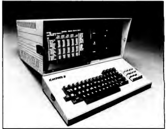
Photo 4: The Kaypro II has the ability to read and write to a variety of disk formats.
