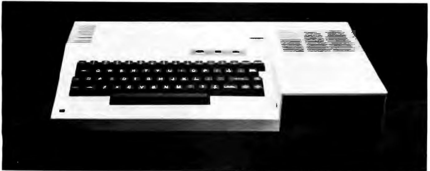
Photo 2: The production version of the Pied Piper computer. The indicator lights for power and disk drives were last-minute additions.
