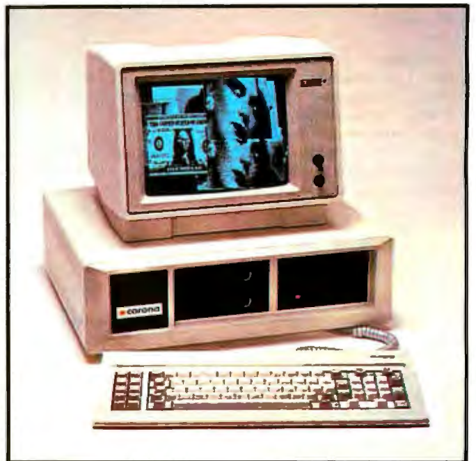
Photo 2: The Corona PC, the desktop version of the Corona portable. The unit shown here has half-height floppy-disk drives, but most units will be shipped with regular-height drives.
