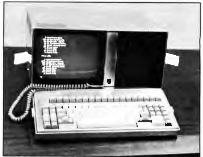
Photo 6: The Starlite HD 20 offers a staggering 20 megabytes of storage in a portable computer.
