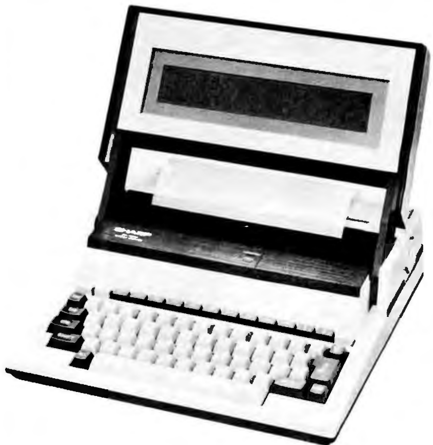
Photo 2: The flip-up 80-character by 8-line LCD screen on the Sharp PC-5000 is only one-third the size of a standard CRT screen.
