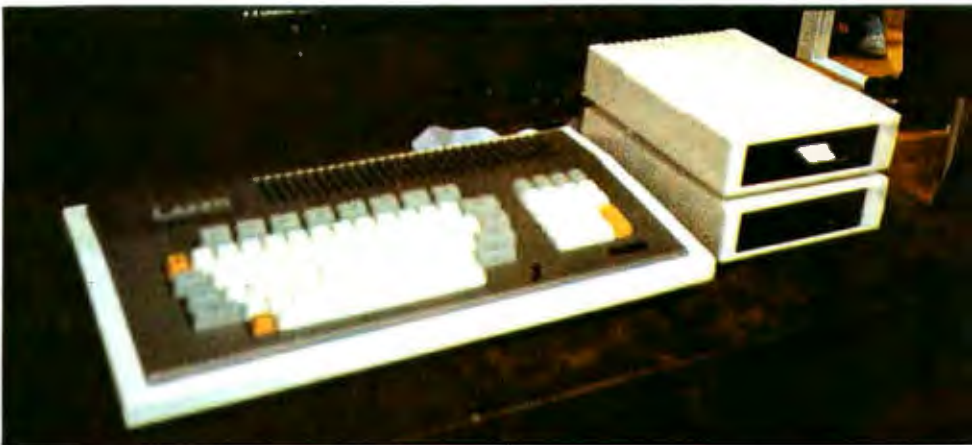
Photo 4: The Laser 3000 from Video Technology, which runs at 2 MHz, was the fastest 6502 machine at the CES Show.
